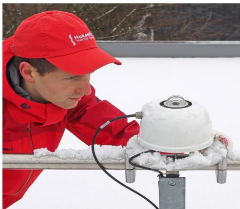
Figure 2 SR22 sensor combined with VU01 ventilation unit.
